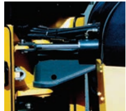
Centerpoint articulated steering with standard crab steer off-set provision.
