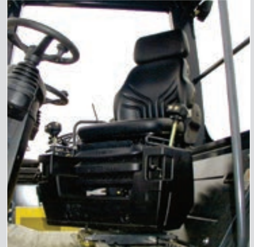
Seat can be moved laterally from side to side or swiveled through 180°.
