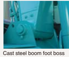
Cast steel boom foot boss
