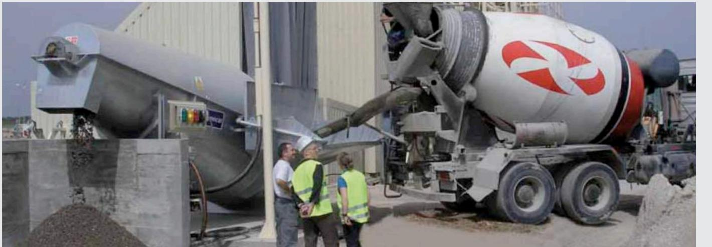
This system incorporates a cone-shaped cleaning vat with an internal spiral that, using an auger screw, rotates to move the material, submerged in water, to the upper part of the cone.
