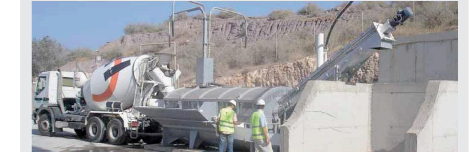
The ECONOR-30 is the recycling model designed for high cleaning demands. It is manufactured as standard with three cleaning showers for positioning three trucks at the same time and it incorporates an exclusive independent area for cleaning vats without waste concrete.
