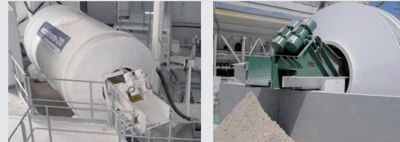
The design of this model is similar to the vat of a concrete mixer truck. The operation, therefore, is also similar. The cleaning spiral that rotates with it is welded inside the vat. The process of movement in contact with water causes sand and cement particles to be separated from the rest of waste material.
