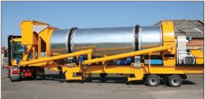
Road towable unit with high efficiency internal lifter design. Optional Insulated and clad drum. Fitted with advanced multi fuel burner. Chassis mounted multi-bank cyclone unit for primary dust collection.
